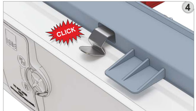
Be sure that the retaining springs are attached to the busbar
